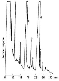
Sterols in the silkworm, Bombyx mori as analyzed with their trimethylsilyl ethers by gas chromatography. An open-tubular glass capillary column (40 m) coated with OV-17 was used at 270  $^{\circ}$ C. Peaks at retention times of 17.0, 19.4, 20.5, 23.6, 24.4 and 25.5 min were assigned by comparison with the authentic samples, to cholesterol (a), campesterol (b), stigmasterol (c), sitosterol (d), fucosterol (e) and isofucosterol (f), respectively.
